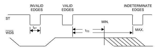
**RESET TIMING DIAGRAM - POWER UP** Figure 12
